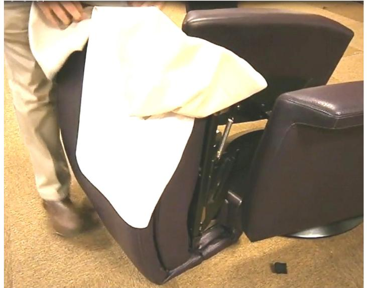
3 Wrap Towels around Back Posts of the Mechanism
