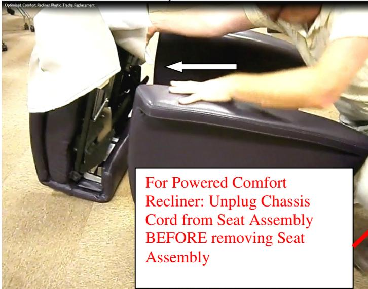
**For Powered Comfort Recliner: Unplug Chassis Cord from Seat Assembly BEFORE removing Seat Assembly**
