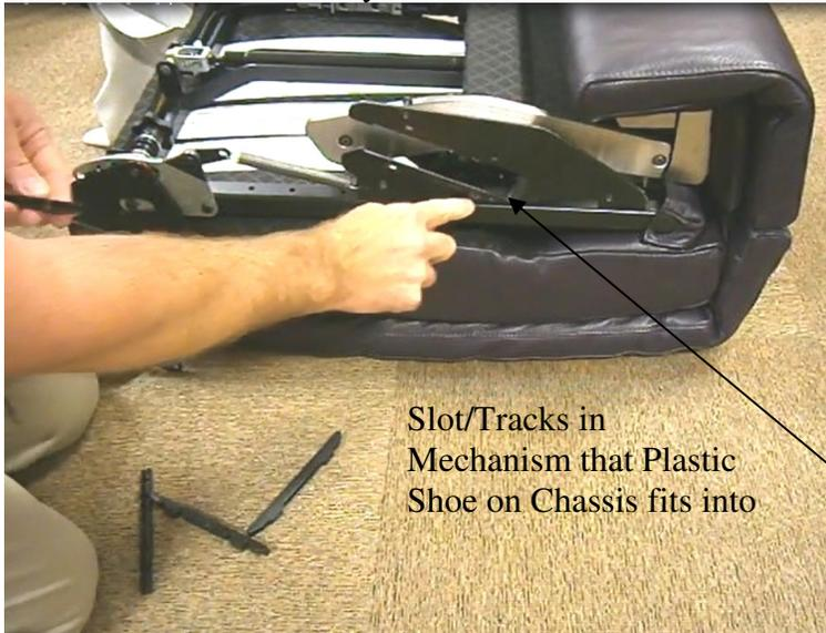
Slot/Tracks in Mechanism that Plastic Shoe on Chassis fits into
