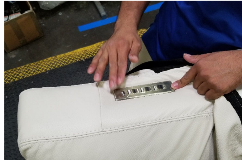
Press the switch into the wooden socket
