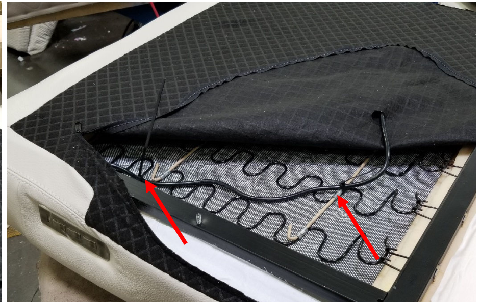
Leave some slack in the cord and zip tie cord to springs in two places as shown. Trim excess tie
