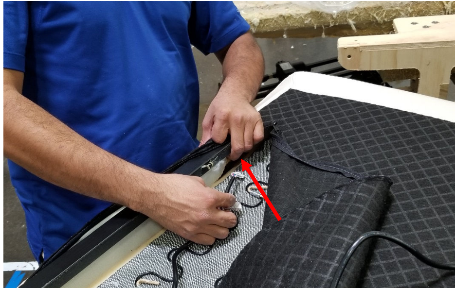
Plug new switch cord into switch through hole in the foam
