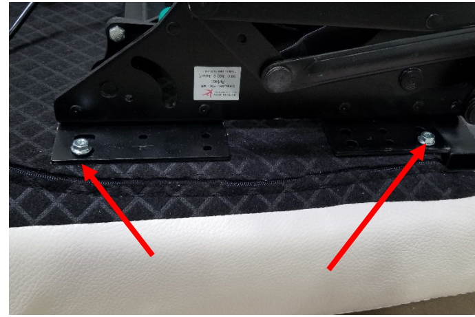
Install 2 nuts on each side of mech
