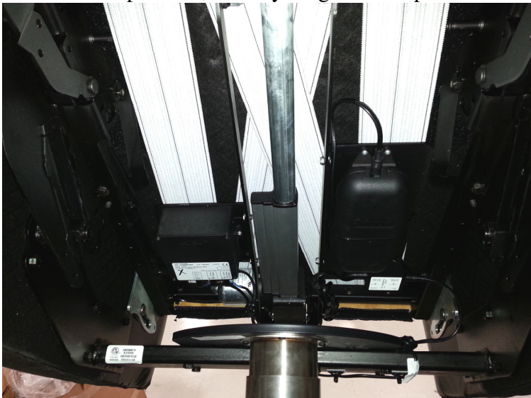
5. To Replace SU04 Box: Remove the two screws/ nylon nuts Holding the Box to the Bracket and replace with the new SU04 Box. Plug in all cords.
